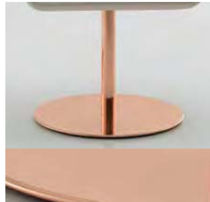
RAME LUCIDO / POLISHED COPPER Trattamento galvanico + verniciatura cataforetica trasparente protettiva antiossidazione e antiditate. Galvanic treatment + protective transparent cathodic dip-paint coating against oxidation and fingermarks. (Minimo 30 pezzi / Minimum 30 pieces)
